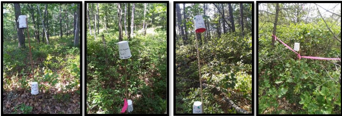
Figure 1. Forest types and climate sensors setting (two iButtons per cup, at 1 m and 0.5 m above the ground). From left to right: Coastal Oak, Oak-Pine, Pine-Oak, Pitch Pine-Scrub Oak.
