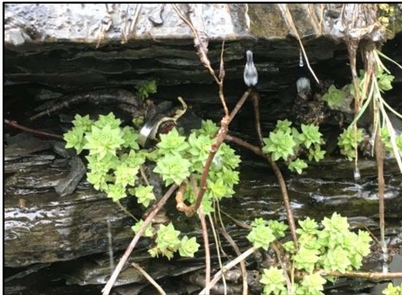
Figure 1. Leedy's roseroot plants in April 2022 with an iButton data logger twist-tied to the basal portion of the plant.
